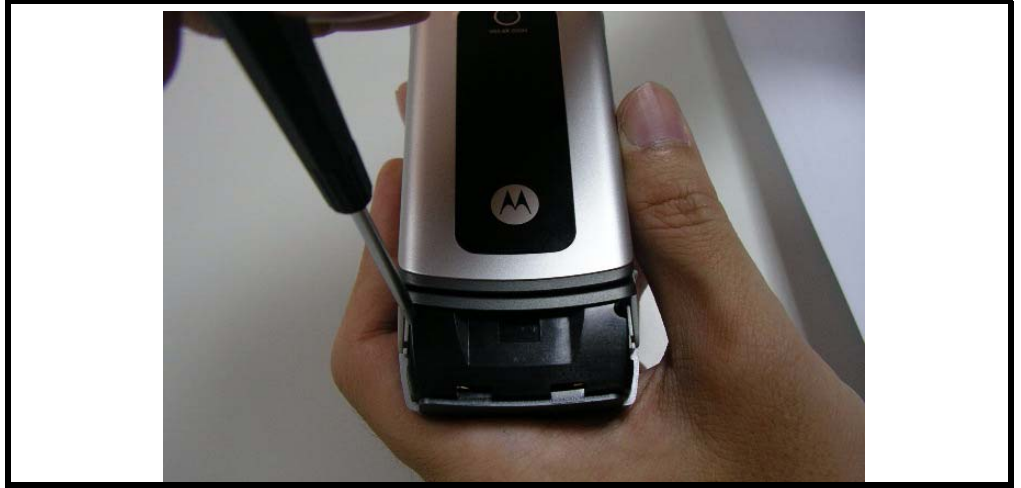
Figure 9. Removing the screws
