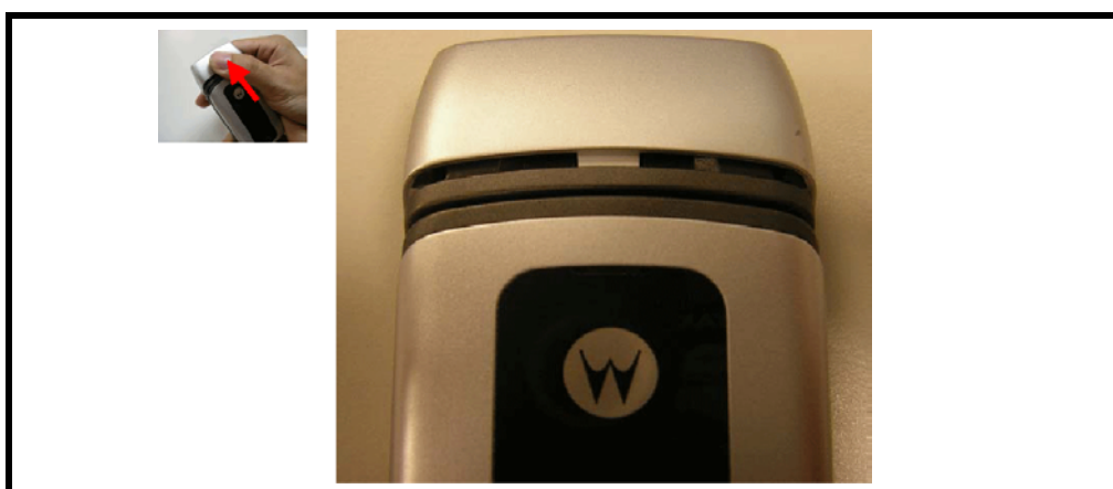
Figure 8. Removing the cap
