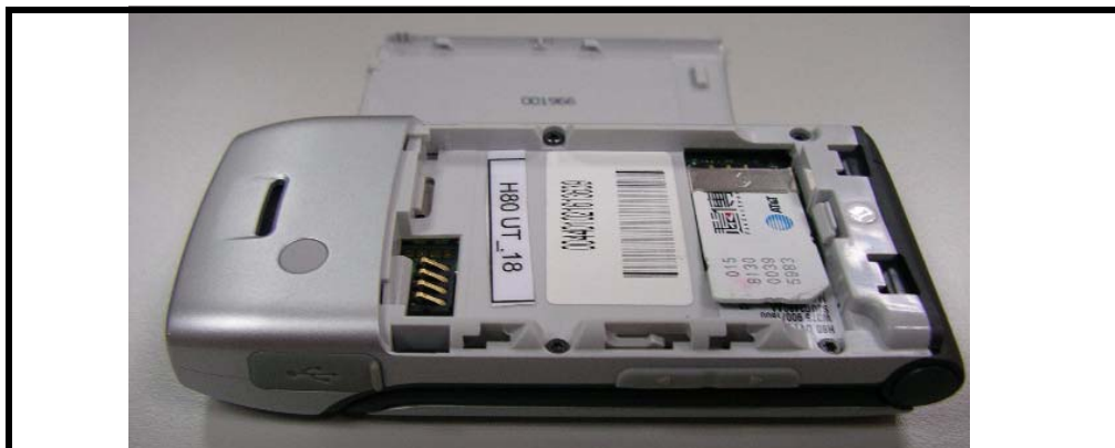
Figure 7. Removing the SIM Card
