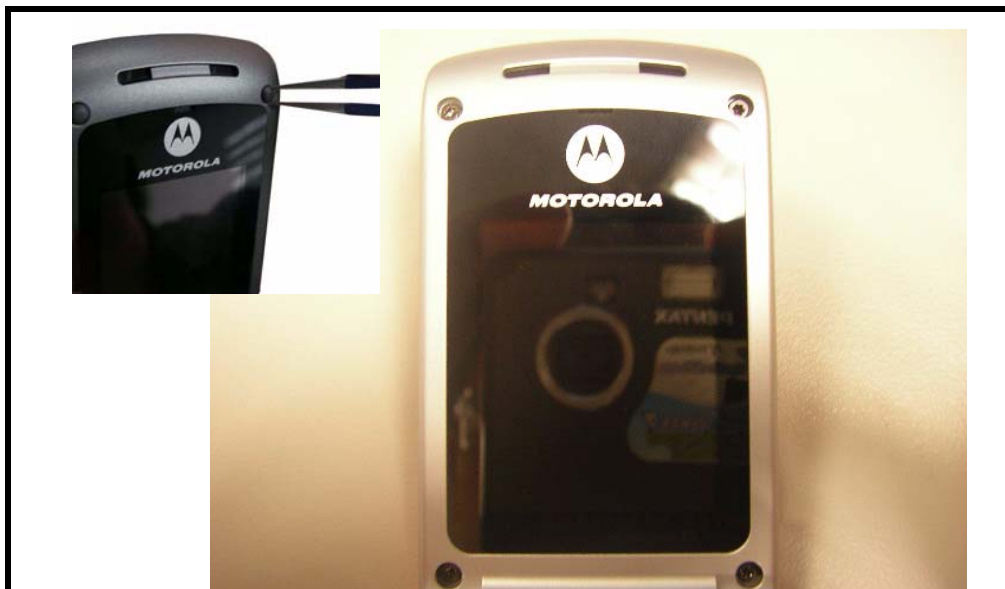
Figure 27. Remove four rubber cover
