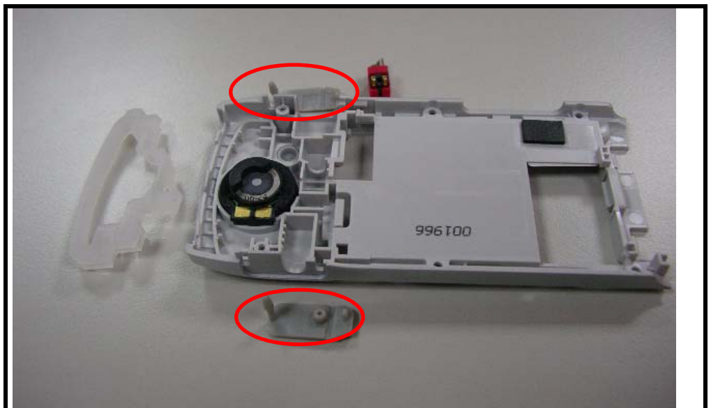
Figure 16. Removing the rubber pad
