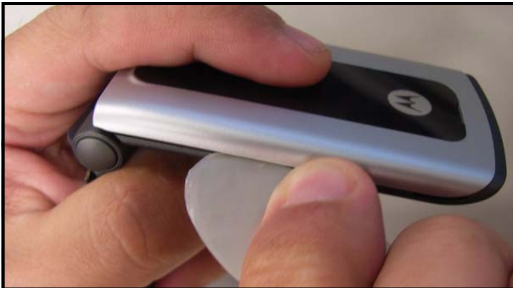
Figure 29. Disconnecting the two halves
