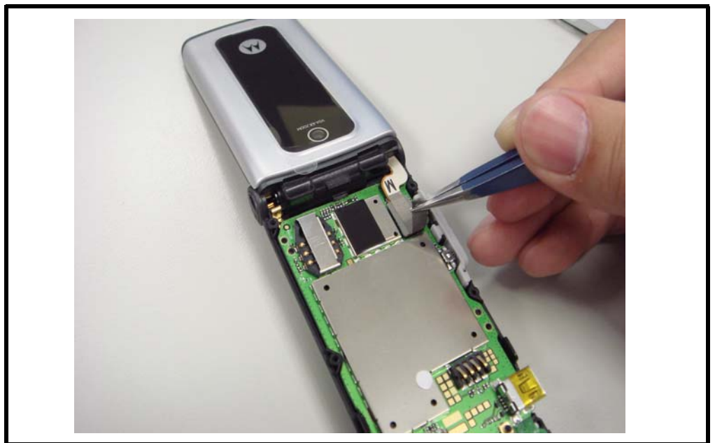
Figure 18. Removing the conduct
