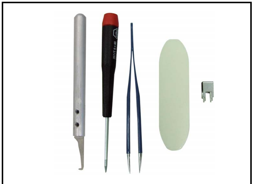
Figure 4. A screwdriver (T5), a pair of tweezers, and a camera jig
