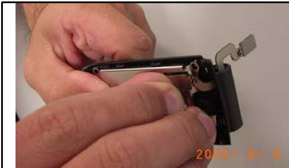
Figure 36. Prying off the FPC connector
