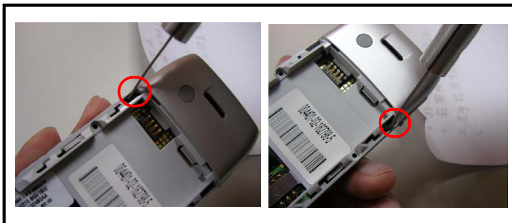
Figure 12. Disengaging the latches
