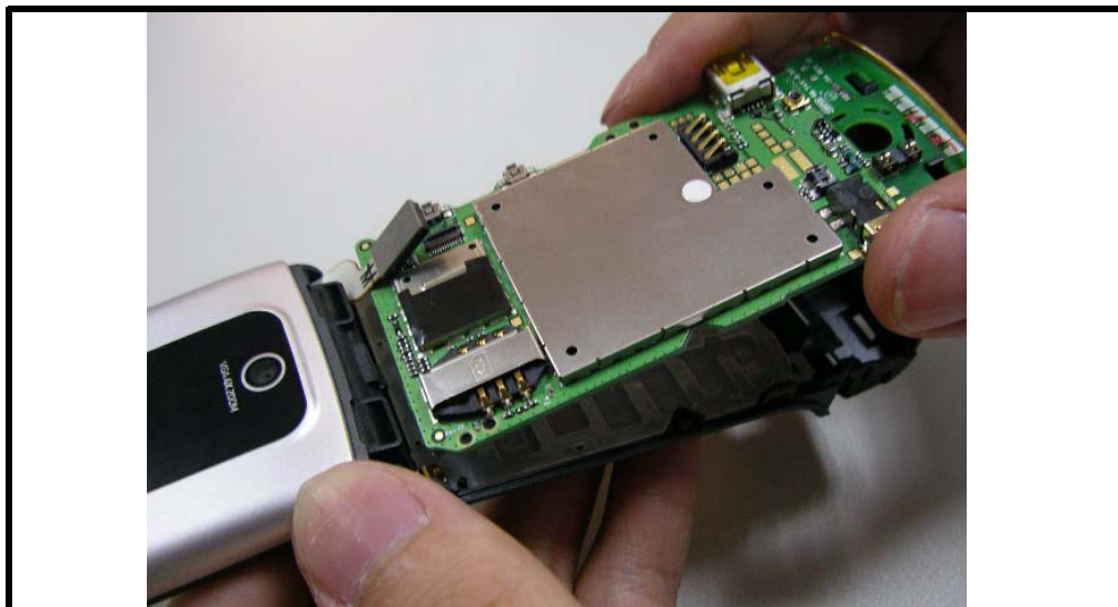
Figure 21. Remove the main board
