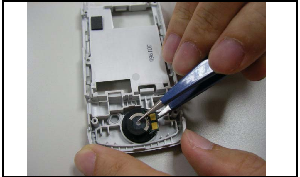
Figure 17. Removing the speaker chip
