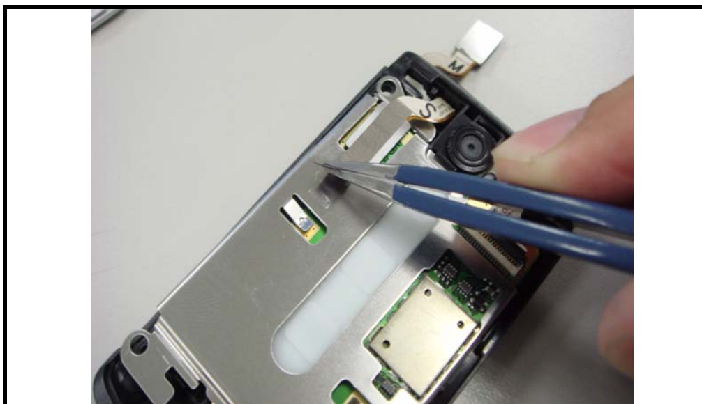
Figure 35. Removing the conduct
