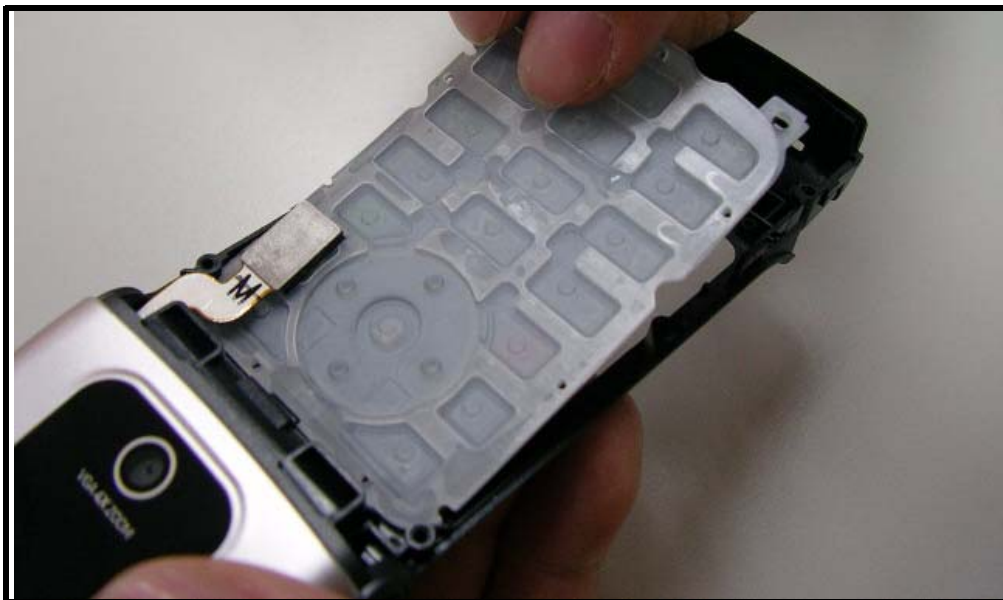
Figure 25. Removing the keypad
