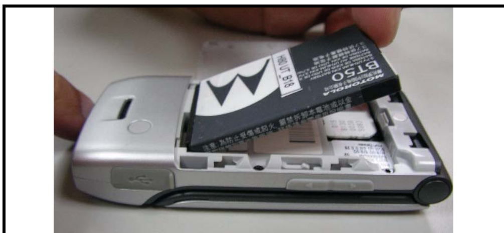
Figure 6. Removing the battery
