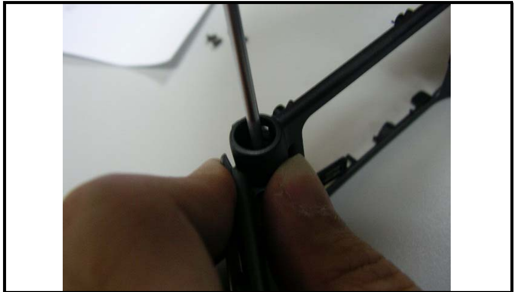
Figure 33. Exerting pressure on the clamshell
