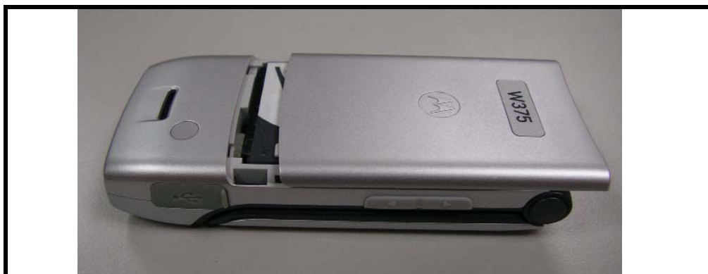
Figure 5. Opening the battery cover
