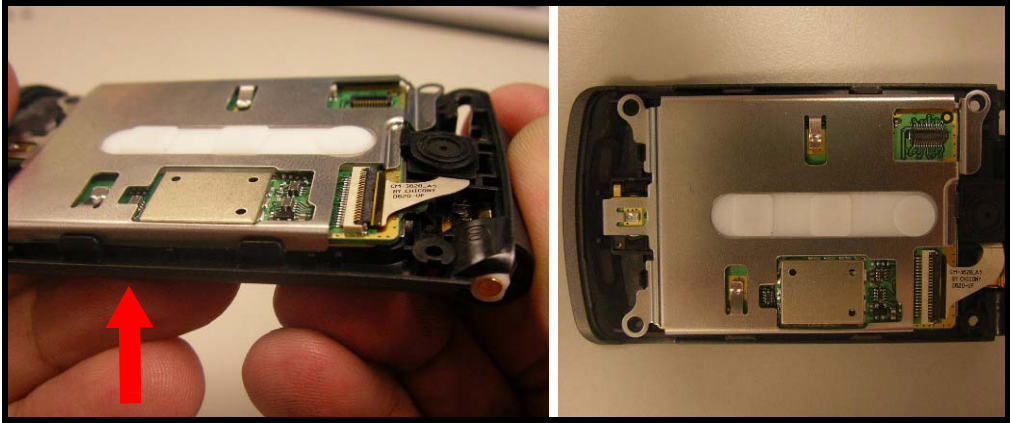
Figure 37. Disengaging the latches
