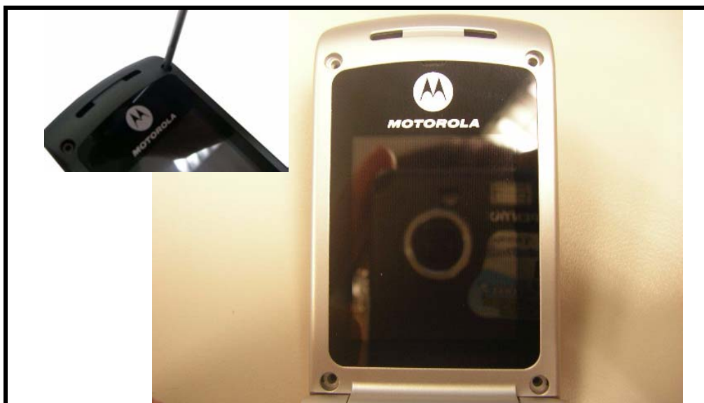
Figure 28. Removing the four T5 screws
