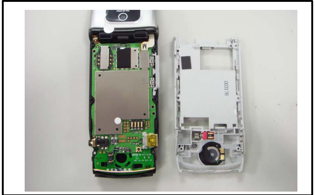
Figure 13. Separating the back housing
